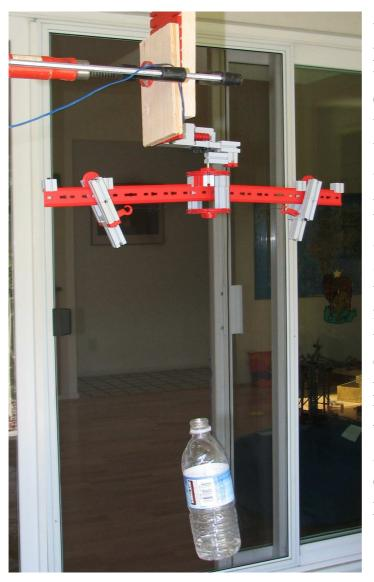
built two small carts that fit on the pole and put them on. Next I tied the thread to the carts. Then I connected the other side of the together and tread added a water bottle. After that I connected the motor to electricity and the pole started to spin. I then added or took away the water from the bottle until the carts went to the outside part of the pole. Next I measured the weight of the water bottle. After that I added weight to the carts and did the same process.
