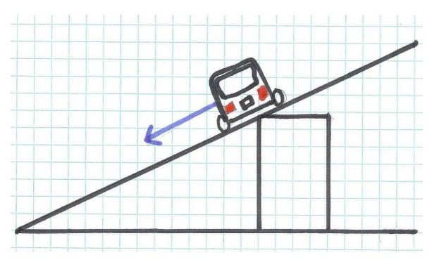
First I built a small car out of Fischer Technik. Then I went outside and placed one side of the board on the bucket, such that the board is tilted. Next I put the plastic table cloth on the board and sprayed water on it. Then I put a car on the board and made the board steeper. I then measured at what point the car would lose grip and slide down the wet
