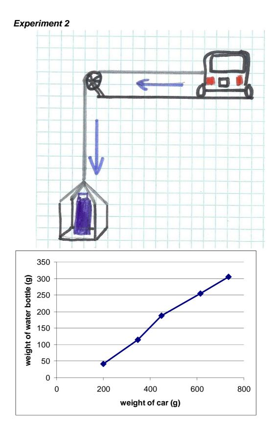
The second experiment I measured the friction force of the car.
