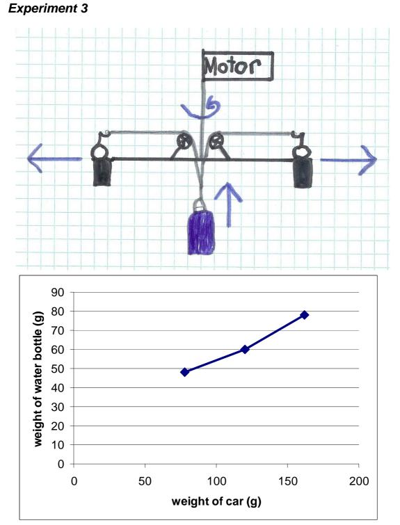
The third experiment I measured the centrifugal force. If the centrifugal force is too big the car will skid.
